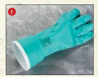
Pull the cuff of the glove over the white ring - insert the narrower end of the ring first.
