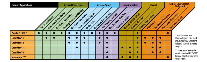
**Pyrolon® CRFR**: A fabric unique to Lakeland that provides Chemical and Flame Resistance, all rolled into one garment. Pyrolon® CRFR provides both Chemical and Flame Resistance and excellent hold out for gasoline, crude oil and many common chemicals found in the Petrochem market. Pyrolon® CRFR is self-extinguishing, won't melt or drip, and meets the NFPA 2113 requirements for section 5.1.9. It is designed to be worn over woven thermally protective coveralls.
