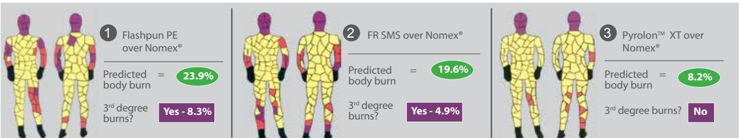
The testing shows that both standard disposables such as Flashpun and FR SMS garments result in higher predicted body burn with very little difference. Only Pyrolon™ garments result in a dramatic reduction in predicted body burn.
