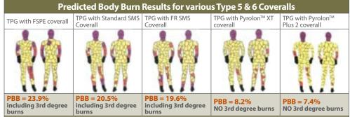
The results show almost no difference between FSP, Standard SMS and FR SMS, with all three producing 2nd and 3rd degree burns. Pyrolon™ Plus 2 and XT coveralls produce much lower predicted burns and no 3rd degree burns
