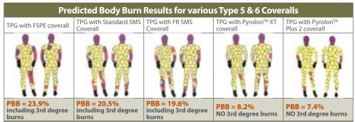
The results show almost no difference between FSP, Standard SMS and FR SMS, with all three producing 2nd and 3rd degree burns. Pyrolon™ Plus 2 and XT coveralls produce much lower predicted burns and no 3rd degree burns
