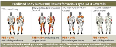
The results show that wearing a standard chemical suit over a TPG not only increases predicted body burn compared against the TPG suit alone, it also results in 3rd degree burns. Wearing a Pyrolon™ chemical suit over the same TPG REDUCES predicted body burn and produced no 3rd degree burns.
