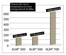
Although all 3 ALM® garments are measured as Class 4. ALM® 700 provides a much higher level of protection - and therefore facilitates greater working times and more protection, than 300/500.
